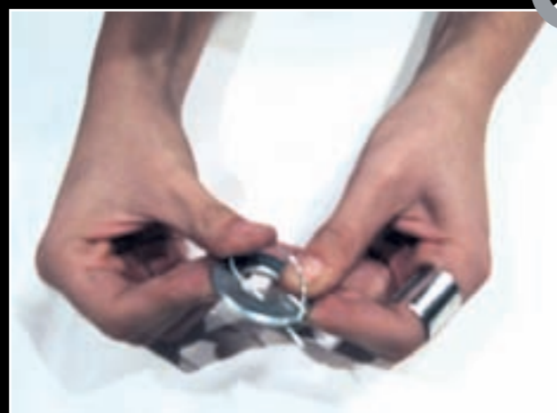
Twist it around one side of the washer. Tighten it with the wire cutter.
